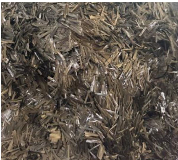
1-rasm. “BASALT HOLDING” MCHJda ishlab chiqarilgan bazalt tolasi (BK-01 marka)
