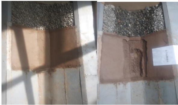
1.2 a,b-rasm. Quyi byefdagi bog'langan grunt eroziyasining boshlanishi
