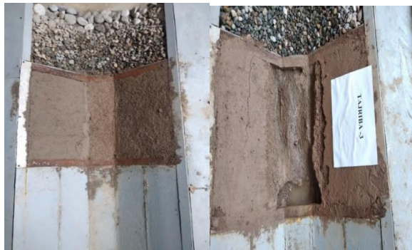
3 a,b-rasm. Elementar dispers zarrachalari yuvilishining dastlabki bosqichi
