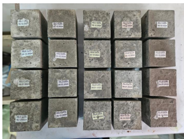
1-rasm. Kimyoviy qo'shimchasiz B30(M400) sinfli betonning 10x10x10 namunalari
